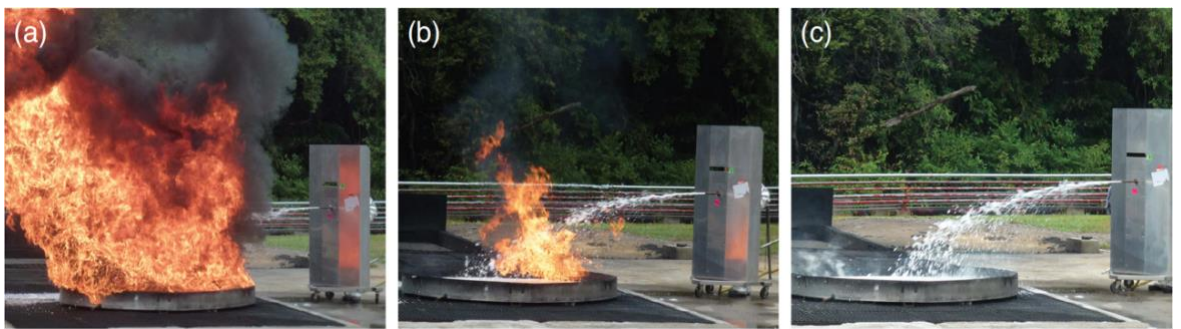
Effective ICAO Level B Fire test demo using C6 AFFF at Singapore Fire Conference, July 2016. (a) pre-burn; (b) ≤C6 AFFF fire control; (c) ICAO Level B ≤C6 AFFF extinguishment
