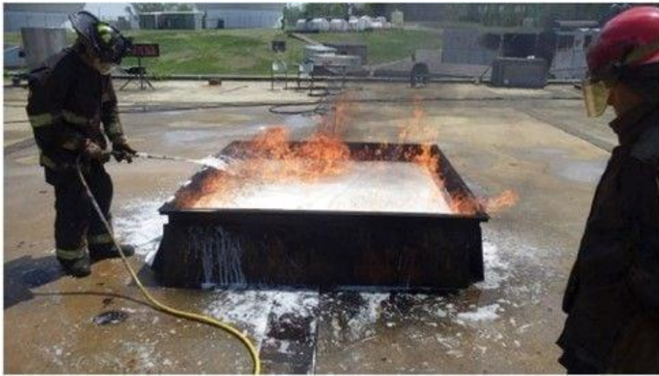
Fig.1: AR-F3 unable to contain gasoline vapours and appearing to react with the foam blanket causing bubbles to break at lower 3-4:1 expansion ratio. 3-4:1 required up to 50% more AR-F3 to extinguish, compared to 7-8:1 expansion ratio use. Reproduced with permission from Fire Protection Research Foundation, Evaluation of the fire protection effectiveness of fluorine free firefighting foams 4 , Copyright© 2020, Fire Protection Research Foundation, Quincy, MA, USA. All rights reserved.
