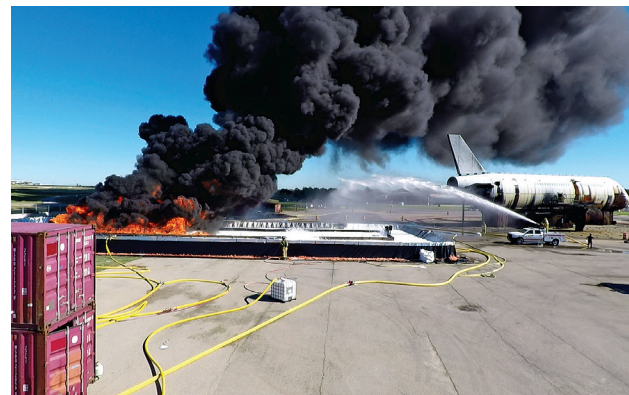
Firefighters spray fluorine-free foam on a hydrocarbon test fire at Dallas Fort Worth Airport.
